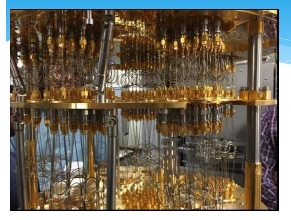
In order to minimize energy loss, the coaxial lines that direct signals between the first and second amplifying stages are made out of superconductors.
