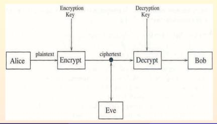
Bob receives the 'ciphertext' and changes it to the 'plaintext' by using a decryption key.
