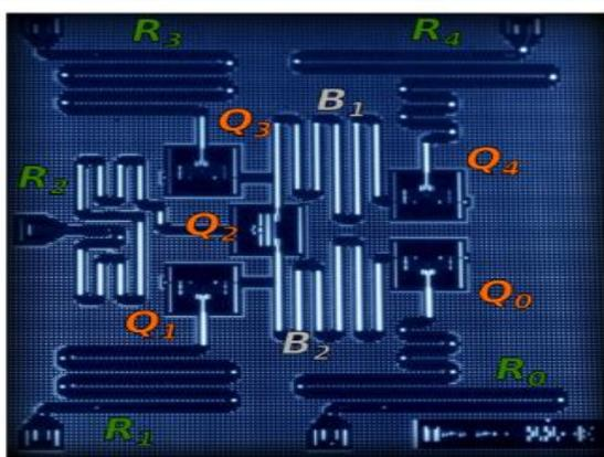
❖ Coupling map = {0: [1, 2], 1: [2], 3: [2, 4], 4: [2]} where, a: [b] means a CNOT with qubit a as control and b as target can be implemented.
