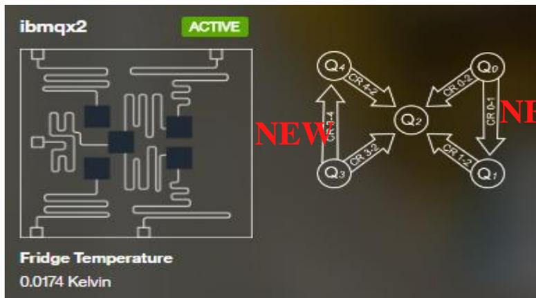
❖ The connectivity is provided by two coplanar waveguide (CPW) resonators with resonances around 6.0 GHz (coupling  $Q_2$ ,  $Q_3$  and  $Q_4$ ) and 6.5 GHz (coupling  $Q_0$ ,  $Q_1$  and  $Q_2$ ). Each qubit has a dedicated CPW for control and readout. This picture shows the chip layout.
