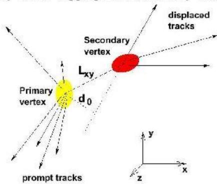
Typical resolution:  $d_0 \sim 30 - 50 \ \mu \text{m}$  or so
