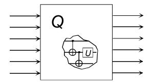
The 2-qubit XOR or "controlled-NOT" gate flips its 2nd input if its first input is 1, otherwise does nothing.
